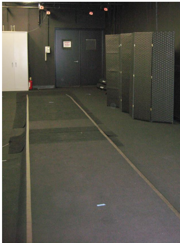
Figure 2-1. Walking platform with two force plates mounted in the center and Motion Analysis camera system setup for motion capture.
